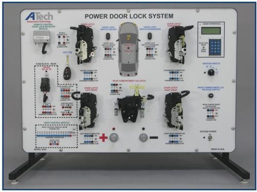
The ATech Power Door Lock Trainer (model 850C) is designed to teach computer and network controlled automotive door lock and theft deterrent system operation. This trainer allows for instructor demonstration, student hands-on reinforcement and troubleshooting practice. Powered by a 12VDC automotive battery or a 12VDC/23A power supply (not included).
