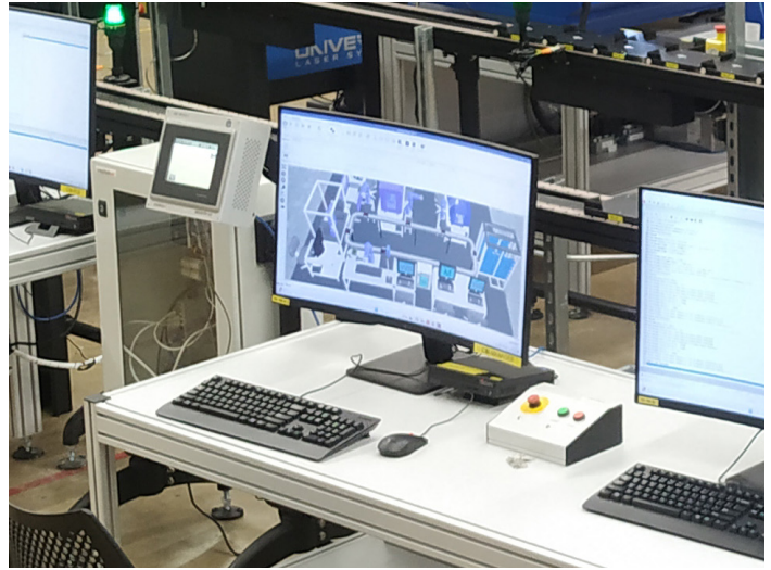
The OpenMES manager includes advanced functionality and digital twinning of the SmartCIM 4.0 process
