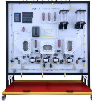
FCU-100V Aircraft Turbine Fuel System Trainer (3 Tank, 2 Engine)
