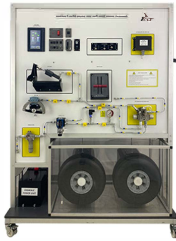
FCU-100V Aircraft Turbine Fuel System Trainer (3 Tank, 2 Engine)
