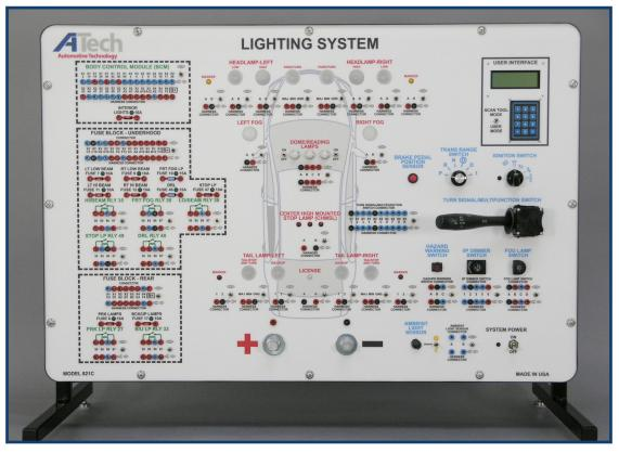
The ATech Lighting System Trainer (model 821C) is designed to teach computer and network-controlled automotive lighting system operation. This trainer allows for instructor demonstration, student hands-on reinforcement, and troubleshooting practice. Powered by a 12VDC automotive battery or a 12VDC/10AMP (minimum) power supply (not included). The Lighting System is based on a CAN platform vehicle.
