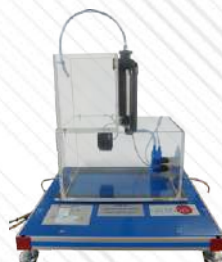
RYC-C. Flow Rate Control Module
