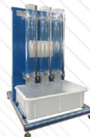
▶ PEDI. Demonstration Infiltration Unit
