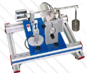
MEMT-3. Dynamic Friction of a Pin on a Disc
