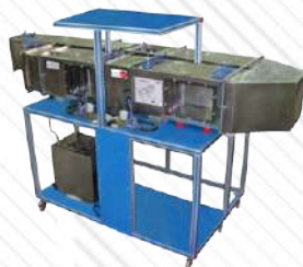
TRAMC/4. Complete Air Conditioning System Model
