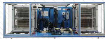
TCREV. Compression Refrigeration Unit with Different Expansion Valves
