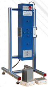
TXC/FF. Free and Forced Convection Heat Transfer Module for TSTCC
