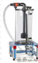
FME04. Orifice Discharge
