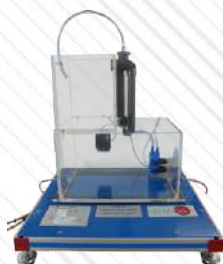
RYC-C. Flow Rate Control Module
