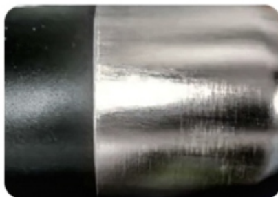
Insulation Cup Paint Removal
